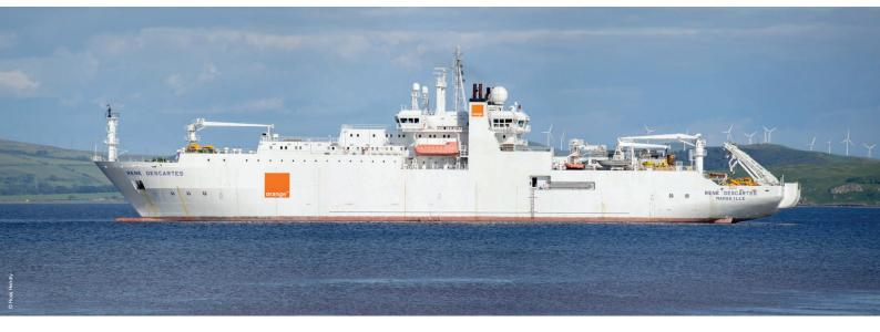
Tailored-built for Orange Marine in 2002, cable ship Descartes is a versatile, high technology vessel, designed to lay and repair submarine fibre optic systems.
